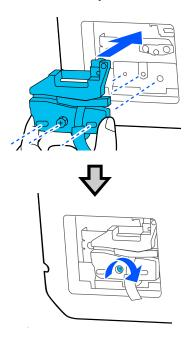
**Note:** Make sure the screw is tightened securely, otherwise the cut position may be slightly shifted or skewed.
