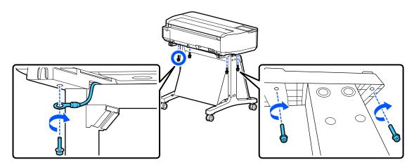
• If your stand includes thumbscrews, insert 4 thumbscrews (2 on each side) into the bottom of the mounting brackets to secure the printer to the stand. On the left rear side, insert the thumbscrew through the wired loop on the printer as shown.
