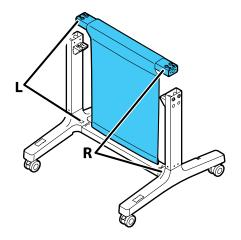
7. Insert 4 screws (2 on each side) into the holes on the paper basket bar to secure it to the legs.
