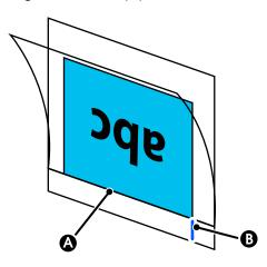
2. Remove the document guide and insert the carrier sheet against the right side of the scanner slot.
