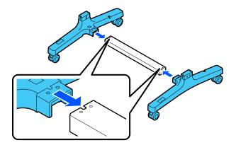
3. Use the Allen wrench to insert 8 screws (four on each side) into the holes on the support brace and leg bases.
