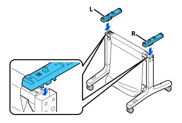
9. Insert 4 screws into 4 screw holders (2 on each side) and insert them into the holes on the legs to secure the mounting brackets.
