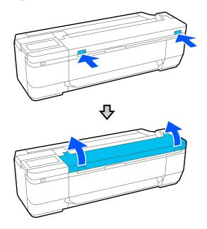
2. Using a soft cloth, wipe off any dust, dirt, or paper particles from the areas highlighted below.
