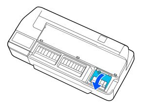
5. Push in the tab at the top of the ink cartridge and pull it out.
