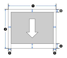
**Note:** Margins may change depending on the **Top/Bottom Margins** setting that you select. The numbers below are the standard settings. If you select **Print Banner** on the printer driver's Layout tab, the top and bottom margins are set to 0.
