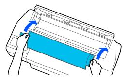
11. Insert the leading edge of the roll paper into the paper feeder until you hear a beep.
