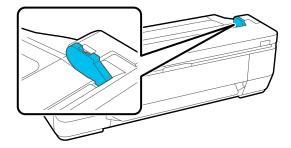
Note: Remove the document guide if you are using a carrier sheet.
