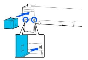
5. Place the used maintenance box in the bag supplied with the new box and seal the bag.
