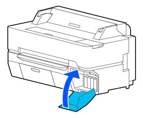
**Caution:** If you remove an ink cartridge for later use, protect the ink supply area from dirt and dust and store it in the same environment as the printer. The valve in the ink supply is designed to contain any excess ink, but do not touch the ink supply port or surrounding area.
