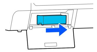
**Note:** Repeat the above procedure for the second maintenance box on the SureColor T5475, if necessary. If you are only replacing one of the maintenance boxes, make sure it is the correct one.
