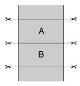
• **Double Cut**: Increases the space between each image and trims each print individually, providing the cleanest edge for borderless printing.
