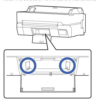
**Note:** You can view the replacement procedure on the LCD screen. Press the ⋒ home button if necessary and select **Settings > Maintenance > Replace Maintenance Box > See Guide**.
