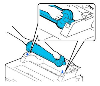
11. Slide the spindle along the spindle holders to fully load the roll.
