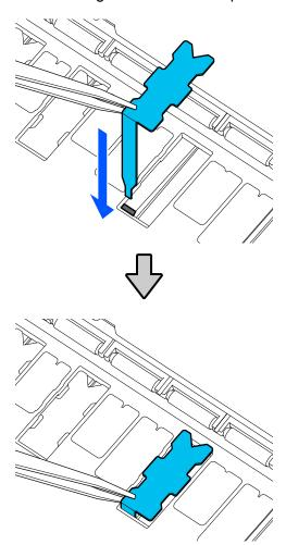
8. Push the protrusions on the sides of the borderless pad into the grooves on the left and right.
