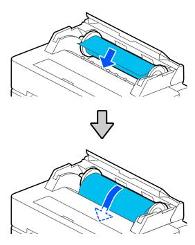
**Note:** Make sure the leading edge of the roll paper is not bent or skewed, or a paper jam or skew error may occur.
