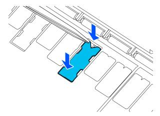
**Caution:** Make sure that no part of the borderless pad extends above the surrounding surface. The borderless pad may rub against the print head and damage it.
