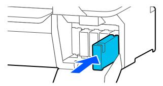
Note: Make sure to insert the cartridge into the correct color location
