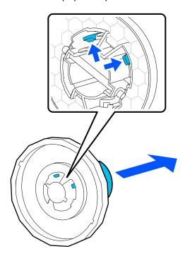
• **3-inch roll core**: Install the 3-inch core adapters on both paper stops. Align the triangle marks on the paper stop with the triangle marks on the adapter and push the adapter in until the tabs are secured.
