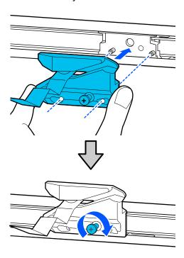
Note: Make sure the screw is tightened securely, otherwise the cut position may shift slightly.
