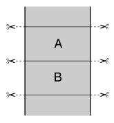
• **Double Cut**: Increases the space between each image and trims each print individually, providing the cleanest edge for borderless printing.
