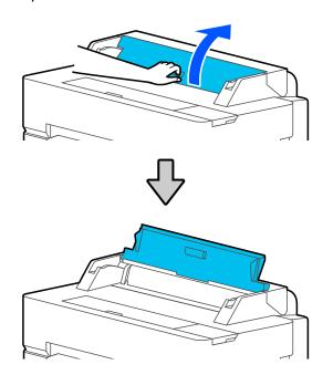
4. Load one sheet of paper, printable side up in portrait orientation. Align the right edge of the paper with the right hand guide on the printer and insert the paper into the printer.
