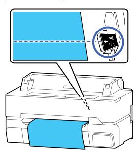
**Note:** You cannot set a cut position further inside than the bottom margin. When the length of paper beyond the cutting position is shorter than the minimum length, the paper will be fed automatically until the minimum length is reached.
