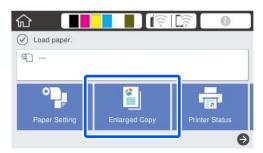
**Note:** If you do not see the **Enlarged Copy** option, make sure the cables connecting the printer and scanner are secure and the scanner is turned on.
