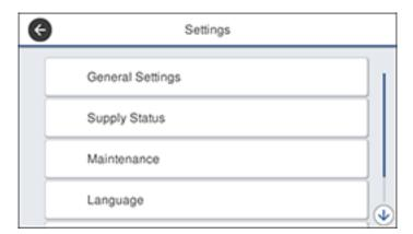
3. Press the up or down arrow to scroll through the menus, or swipe up or down on the LCD screen.
