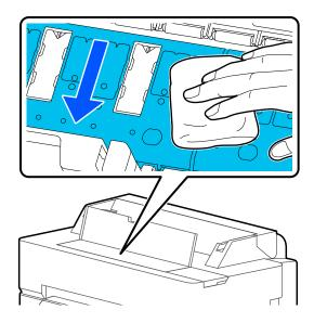
**Note:** For stubborn dirt, dampen a soft cloth with neutral detergent and wring it out, then clean the platen as shown above. Dry the platen with a soft, dry cloth when you are finished.
