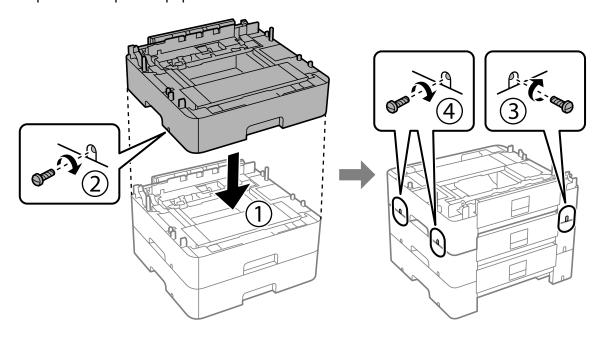
8. Lift up your product and gently lower it onto the paper cassette unit with the corners aligned. Secure the product to the paper cassette unit using the included screws.
