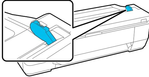
**Note:** Remove the document guide if you are using a carrier sheet.
