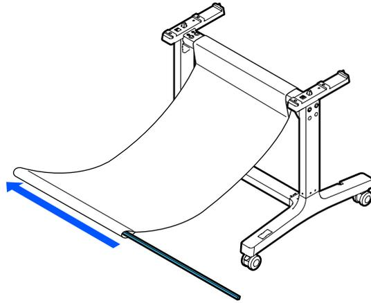
11. Insert the top of the paper basket support rods through the loops on the paper basket cloth and attach them to the paper basket rods.
