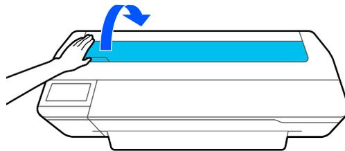
2. Release the central lock and open the roll paper cover.
