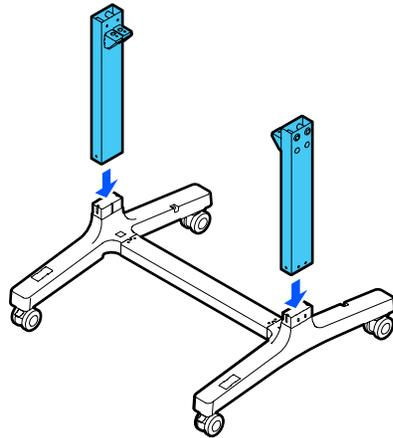
5. Insert 8 screws (4 on each side) into the holes in the legs.
