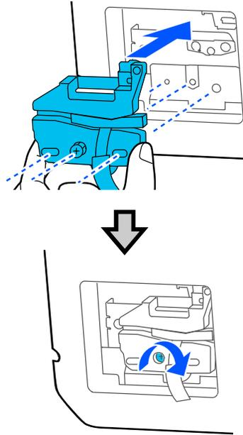
**Note:** Make sure the screw is tightened securely, otherwise the cut position may be slightly shifted or skewed.
