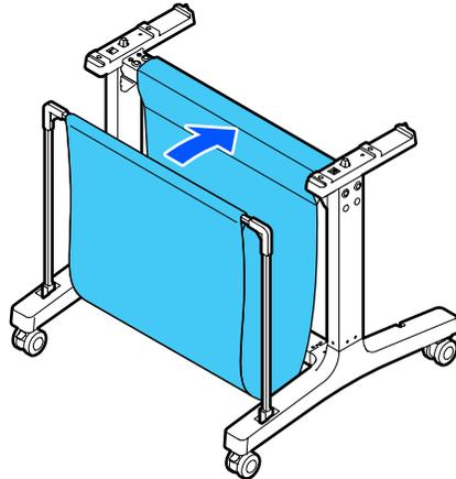
14. On the back of the paper basket and stand, attach the loops on the paper basket cloth to the hooks on the leg bases as shown.
