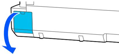
2. Pull out the maintenance box carefully without tilting it.
