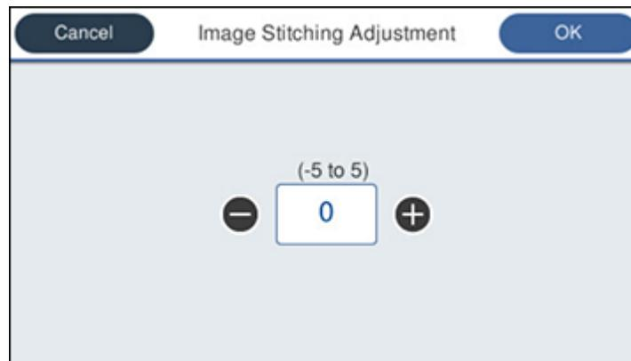
3. Tap the adjustment value area to adjust the value directly, or use the +/- buttons to change the value. Shifting the value of the adjustment by 1 will correct the misalignment by approximately 0.1 mm.
