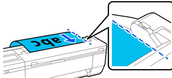
3. Support the original with both hands and insert the top edge into the scanner slot until it is automatically moved to the scanning position. You will hear a beep when loading is complete.
