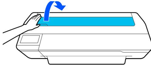
4. Load one sheet of paper, printable side up in portrait orientation. Align the right edge of the paper with the right mark line and plastic ledge on the printer and the left mark line for the paper size you are using.
