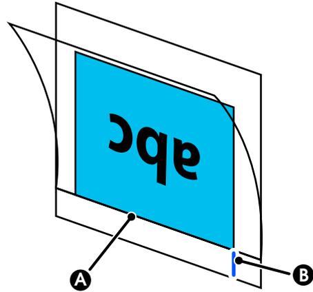
2. Remove the document guide and insert the carrier sheet against the right side of the scanner slot.
