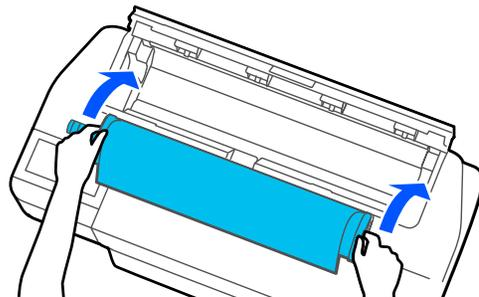
11. Insert the leading edge of the roll paper into the paper feeder until you hear a beep.
