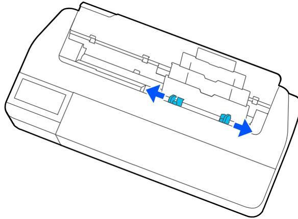
6. Load paper, printable side up, into the auto sheet feeder.
