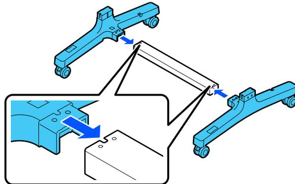
3. Use the Allen wrench to insert 8 screws (four on each side) into the holes on the support brace and leg bases.
