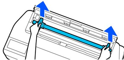
6. Remove the transparent paper stop from the spindle.
