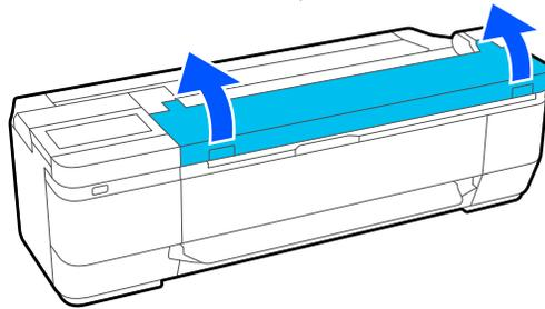
2. Using a soft cloth, wipe off any dust, dirt, or paper particles from the areas highlighted below.
