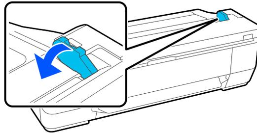
When you are done scanning, remember to re-install the document guide on the printer.
