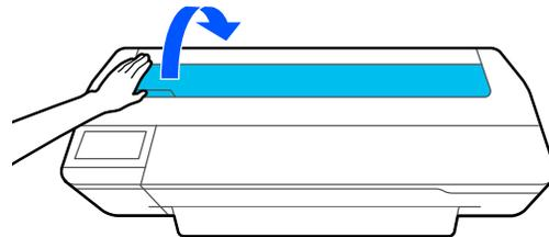
4. Tilt back the auto sheet feeder and pull the paper support extensions all the way out and upward.
