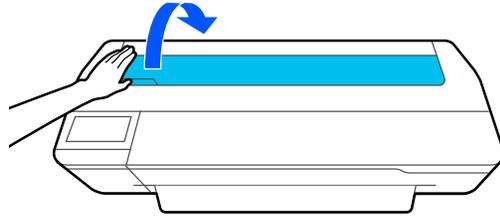
4. Release the central lock and open the roll paper cover.
