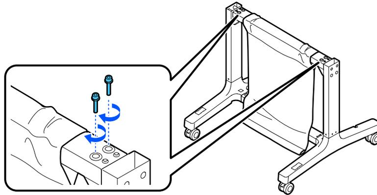
8. Make sure the L and R stickers on the mounting brackets are correctly oriented with the left and right legs and attach them as shown.
