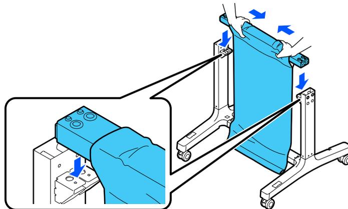
**Note:** Make sure the L and R stickers on the paper basket bar are correctly oriented with the L and R stickers on the leg bases.
