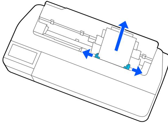
2. Fold down and push in the paper support extensions and close the auto sheet feeder.
