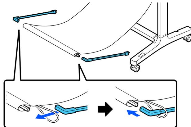
12. Insert the ends of the paper basket support rods into the holes on the leg bases.
