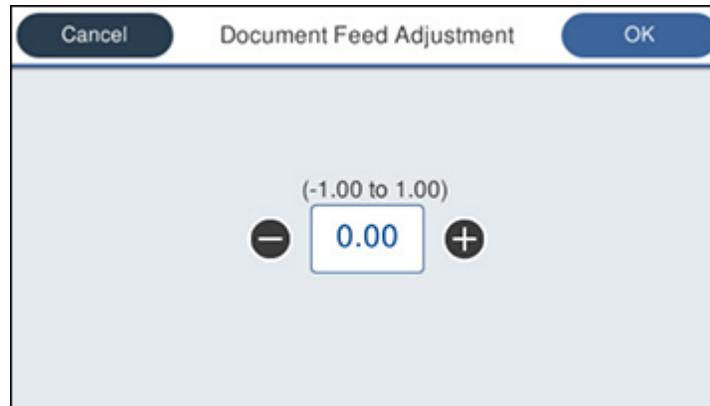
3. Tap the adjustment value area to adjust the value directly, or use the +/- buttons to change the value.
