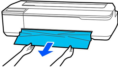
6. Open the front cover and remove any other jammed paper as necessary.
