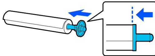
9. Attach the transparent paper stop to the spindle and press it in until there is no gap between the paper stop and the roll paper.
