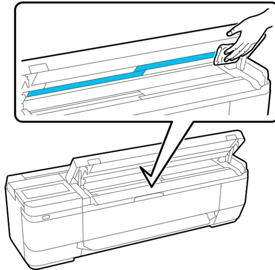
**Caution:** Do not apply excessive force to the glass surfaces. Do not use brushes or hard objects; they may scratch the glass and affect the scan quality. Do not spray glass cleaner directly onto the glass surface.
