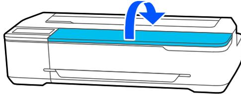
4. Press the tab on the ink cartridge cover and lift to open the cover.
