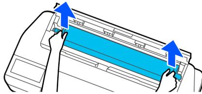
5. Remove the transparent paper stop from the spindle.
