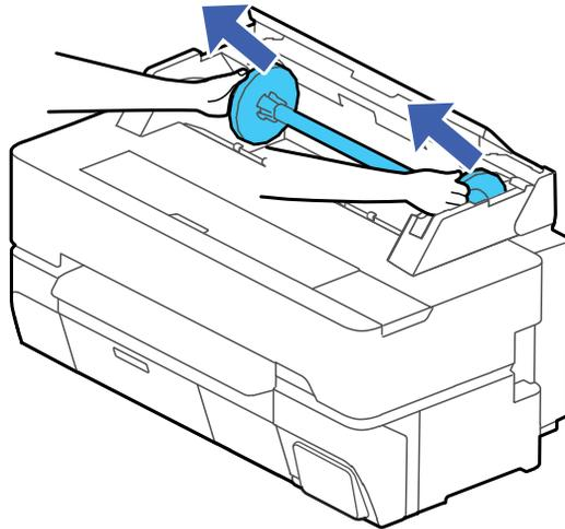
5. Remove the transparent paper stop from the spindle.
