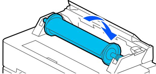
12. Insert the leading edge of the roll paper into the paper feeder until you hear a beep.
