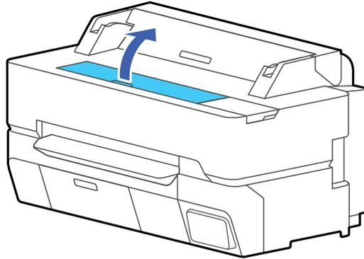
4. Use a soft cloth to remove dust and dirt from the platen. Thoroughly clean the area shown in blue in the image below. Wipe from the inside to the outside of the platen to clean it as shown here.
