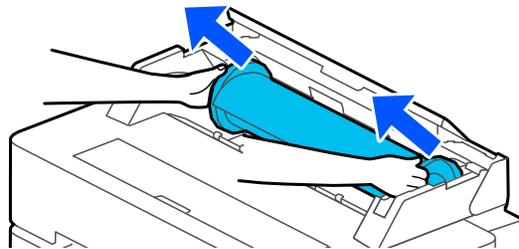
4. Remove the transparent paper stop from the spindle.
