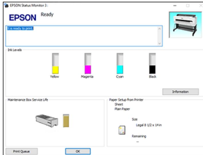
2. Replace or reinstall the ink cartridge or maintenance box as indicated on the screen.
