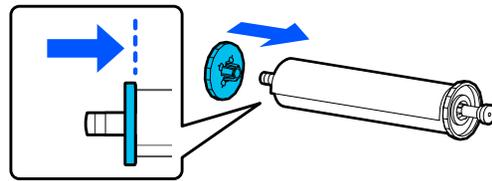
10. Place the roll paper into the spindle holders with the black end of the spindle on the right.
