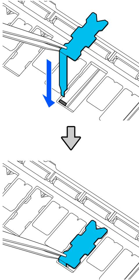
8. Push the protrusions on the sides of the borderless pad into the grooves on the left and right.
