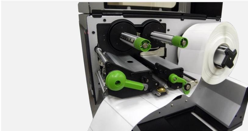
4. Thread the leading edge of the label forward through the media guide bar pass media sensor, and place the leading edge onto the platen roller.
