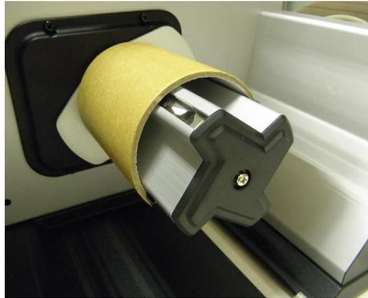
4. Install the paper core onto the liner rewind spindle then open the peel-off roller release lever.
