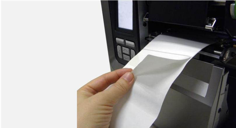
2. Open print head release lever and label guide bar release lever, then pull approximately 650mm of label through the front of the printer.
