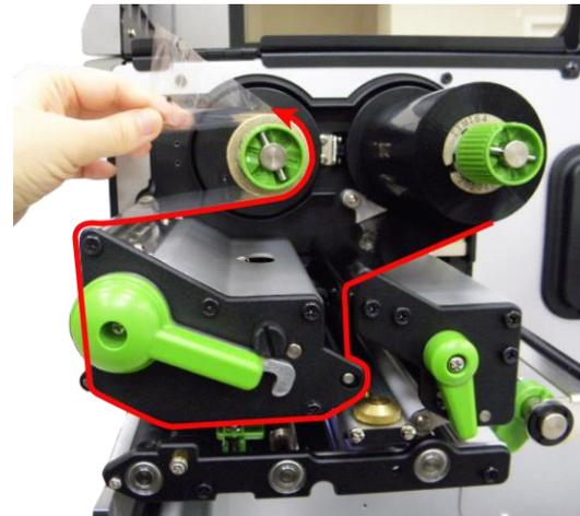
4. Thread ribbon below the ribbon guide bar through ribbon sensor slot.
