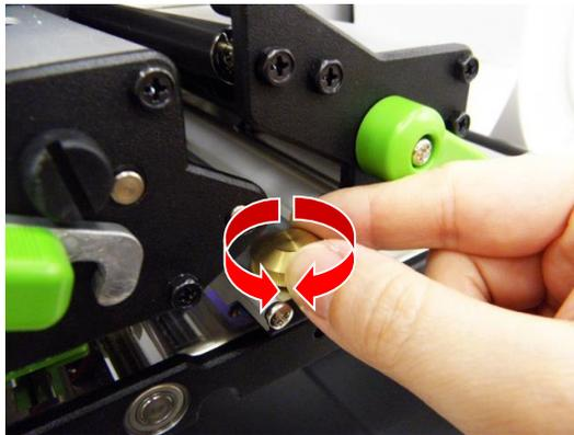
**7.** Move the media sensor by adjusting the media sensor position adjustment knob, make sure the gap or black mark sensor is at the location where media gap/black mark will pass through for sensing.
