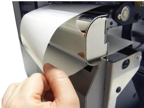
3. Open print head release lever and label guide bar release lever to pull approximately 650mm of label through the front of the printer.
