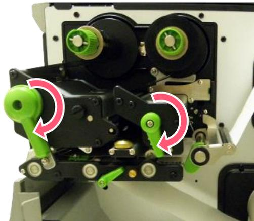
8. Close print head release lever and label guide bar release lever.
