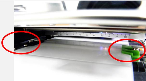
**6.** Adjust the front label guide (green) to fit the label width.
