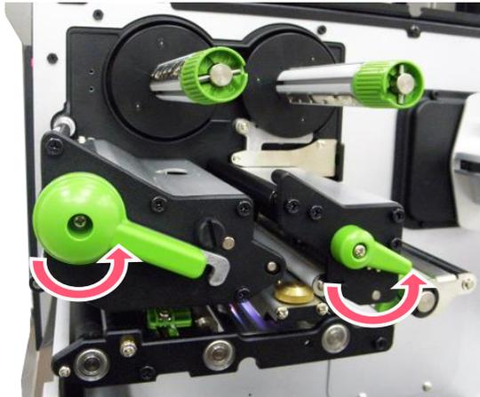
3. Open the print head release lever and label guide bar release lever for loading media.
