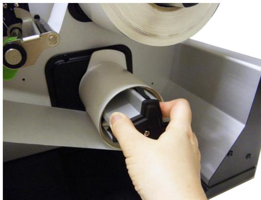
6. Wrap the liner onto the paper core and wind the spindle until the liner stretched properly.
