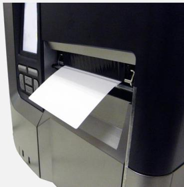
9. Press the FEED button to test.
