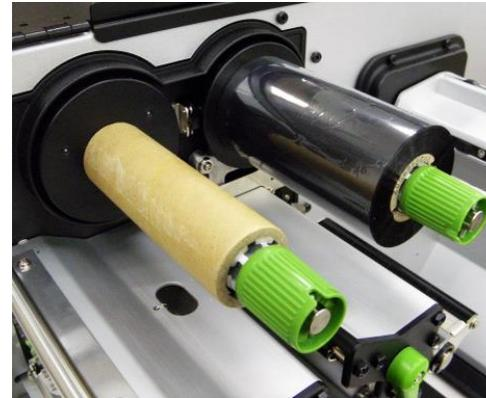
2. Install ribbon on the ribbon supply spindle and paper core on the ribbon rewind spindle.
