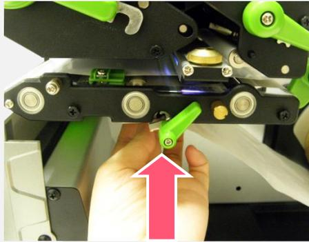
7. Press the middle of the peel-off roller to close the peel-off roller release lever.
