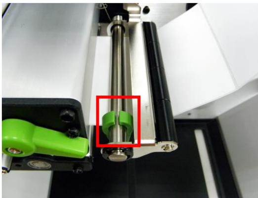
5. Adjust the rear label guide to fit the label width.
