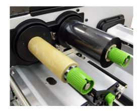
Install ribbon on the ribbon supply spindle and paper core on the ribbon rewind spindle.
