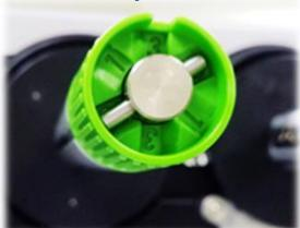
**Ribbon Supply Spindle Tension # 2**
