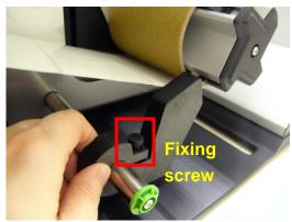
**6.** Adjust the supply holder guide to fit the supply width. Turn the screw to fix the supply holder guide.
