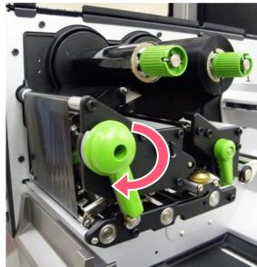
Close the print head mechanism and the lever.
