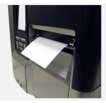
**9.** Press the FEED button to test.
