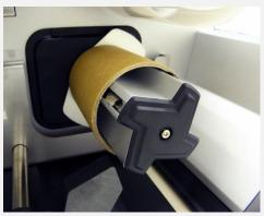
2. Install the paper core on the rewind spindle.
