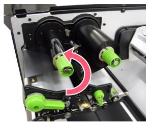
Wind the ribbon rewind spindle counterclockwise until the ribbon is smooth, properly stretched and wrinkle-free.
