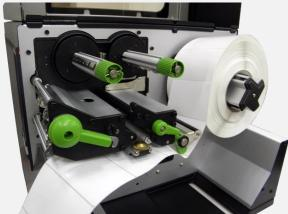
4. Thread the leading edge of the label forward through the media guide bar pass media sensor, and place the leading edge onto the platen roller.
