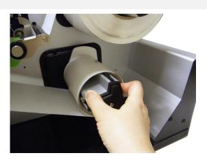
**4.** Install the paper core onto the liner rewind spindle then open the peel-off roller release lever.
