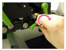
**5.** Feed the leading edge of liner through the peel-off sensor and peel-off roller.
