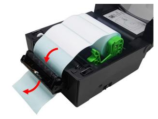
**8.** Close the printer's top cover. Set the print mode to Peeler Mode and then print a label to check if the peel module works well. For how to set the print mode to Peeler Mode, please refer to 6.7 Configuring Optional Kits and 7.1.1 TSPL.
