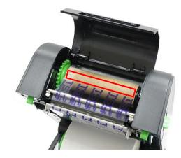
**9.** Rotate the gear in the indicated direction until the ribbon completely covers the printhead.
