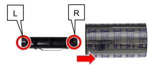
6. Repeat the procedures described in step 4 to load the ribbon into its compartment.
