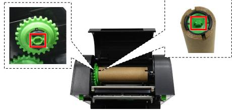
**5.** Orient the core adapter as indicated and then insert the core adapter into the ribbon core.
