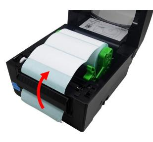
6. Thread the media through the opening on the peel module.
