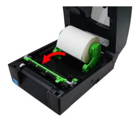
**7.** Press the media guide adjustment button to move the media guides until the guides fit the width of the media.
