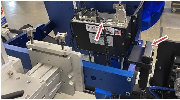
3. Inspect the system to ensure that product hopper, label applicator, and wrap belt assembly are not contacting the any part of the conveyor rollers. Ensure the system guarding is in place, and is not contacting the conveyor rollers.
