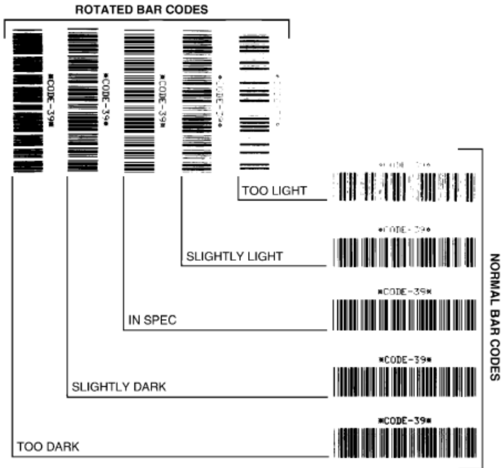
Figure 10 Barcode Darkness Comparison
