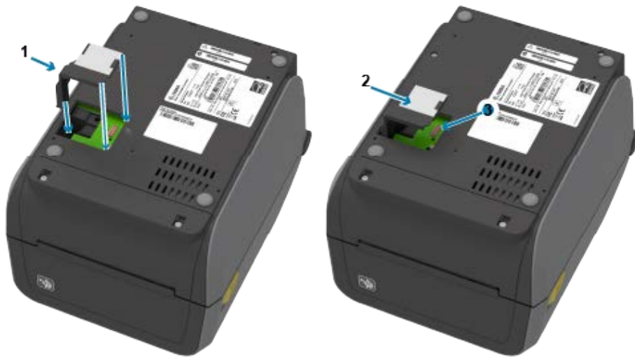
Figure 3 Seating the Module (steps 4–6)
