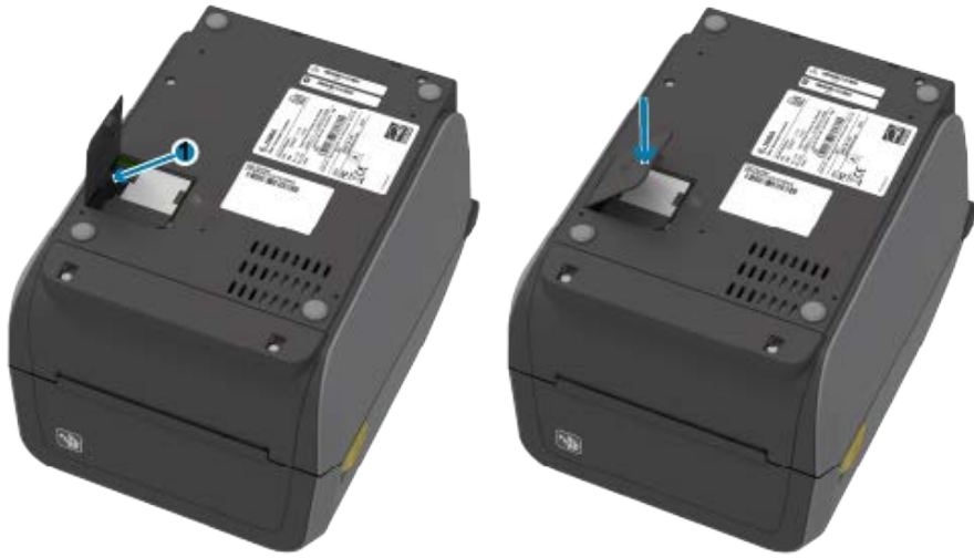
Figure 4 Closing the Wireless Connectivity Door (steps 7–9)
