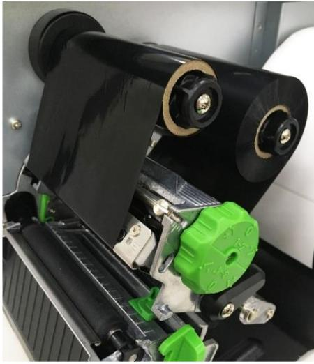
6. Wrap the ribbon onto the rewind spindle. Keep the ribbon flat and without wrinkles.
