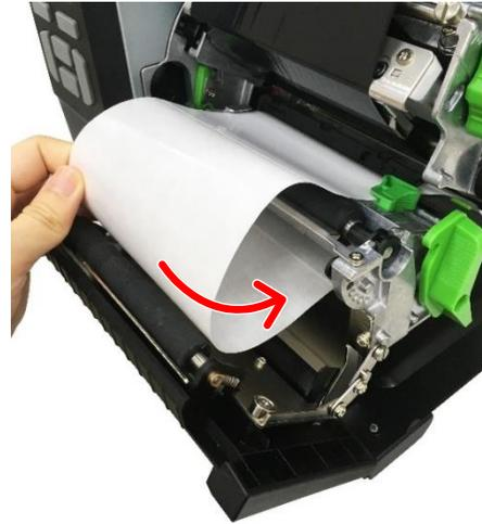
9. Feed the leading edge of liner through the peel-off module slot as indicated.
