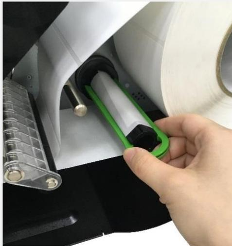
10. Pull out the securing clip (green). Wind the liner onto the spindle until the liner stretched properly.
