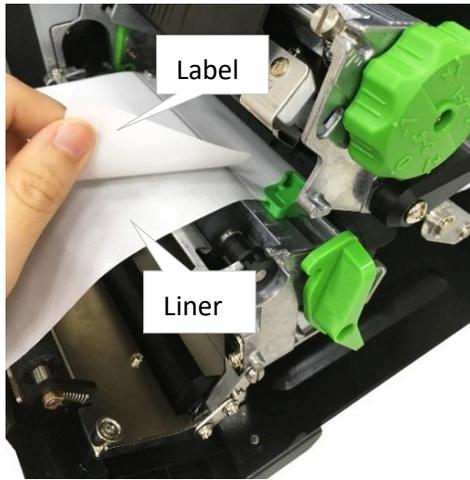
7. Release the lever to open the printhead after calibrating. Release peel-off module lever.
