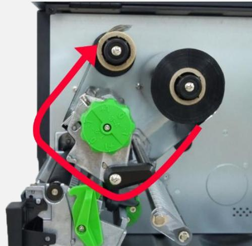
5. Thread the ribbon through the open space between printhead and platen roller. Then pull the ribbon onto the paper core.
