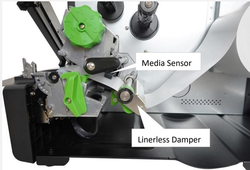
3. Refer to [Loading the Media](#) section to thread the media under the damper, through the media sensor and under the printhead. Keep feeding the media until the media extends out of the front side of the linerless cutter (or tear) module.
