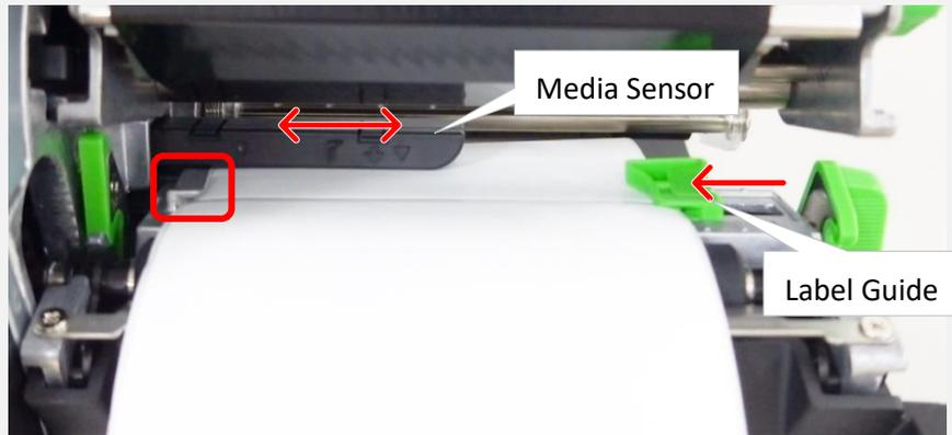
4. Adjust the position of the media sensor and the label guide to fix the media position.
