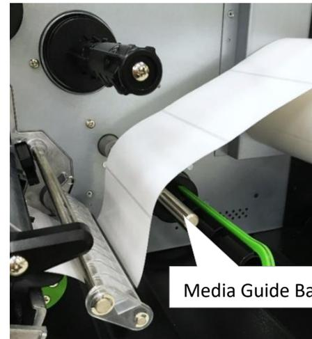
3. Install the label as indicated. (Pass the label over the top of guide bar and under the damper, through media sensor, and label guide.)
