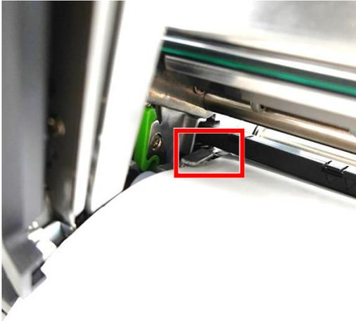
4. Align the media with the media guide ensuring that the media is threaded under the guide.
