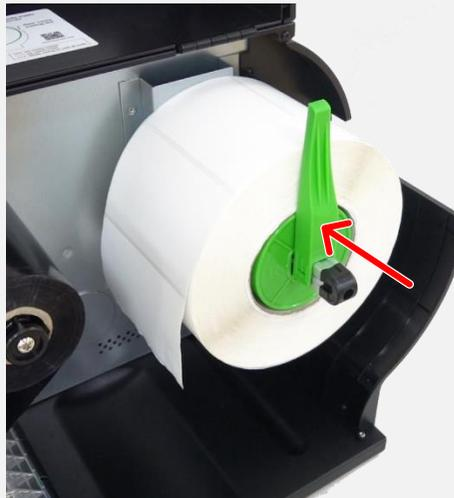
4. Flip the label roll guard up and push it to fit the width of label roll.
