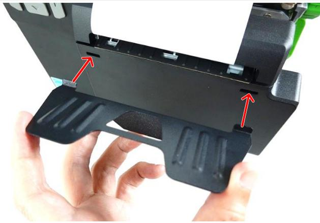
10. (For cutter module only) Insert the ribs on the label tray into its corresponding opening on the front panel of the cutter module.
