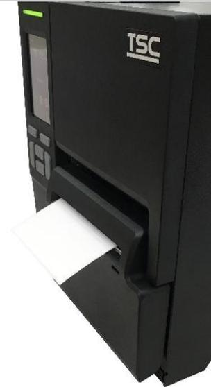
3. Close the printhead and the cutter module.
