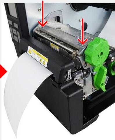
6. Close the upper bar for the linerless cutter (or tear) gate.
