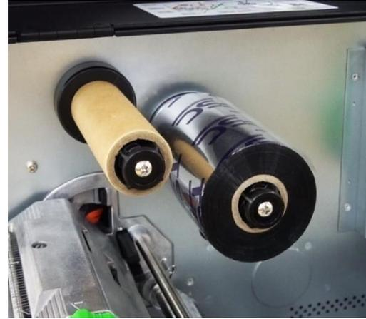
2. Slide the ribbon onto the ribbon supply spindle until it is flush with the flange.
