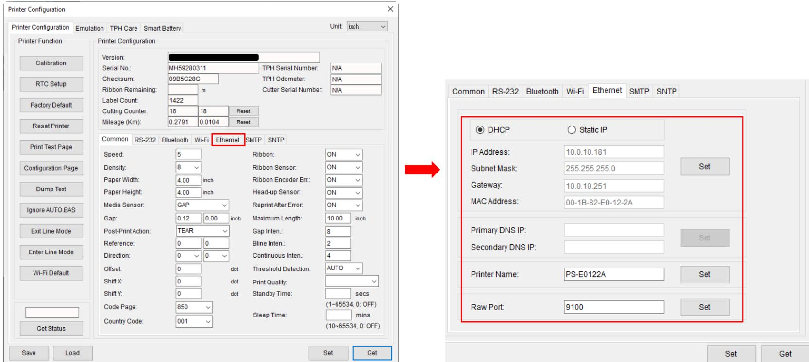
The image shows two screenshots of the printer configuration interface. The left screenshot shows the 'Printer Configuration' dialog box with the 'Ethernet' tab selected. The right screenshot shows the 'Ethernet' configuration page with the 'DHCP' option selected and the 'Set' button highlighted.
