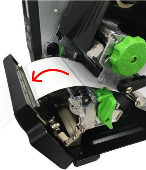
1. Open the media cover, the printhead, and the cutter module.
