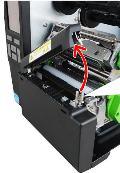
2. Open the upper bar for the linerless cutter (or tear) module gate.
