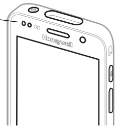
Battery Status LED
