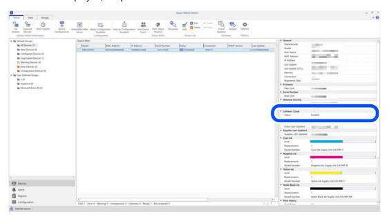
• If "Disabled" or an error number is displayed, the printer registration has failed. Check the solutions listed in "Error Number List (Only for CW-C8000 Series)" on page 26. In this example, the error number is 910005.
