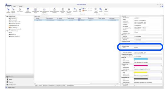
• If "Disabled" or an error number is displayed, the printer registration has failed.
