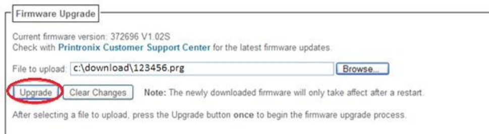
Figure 5 Uploading Firmware File for Upgrade
