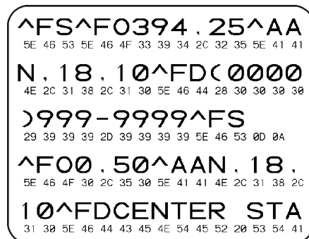
Figure 16 • Communications Diagnostics Test Printout
