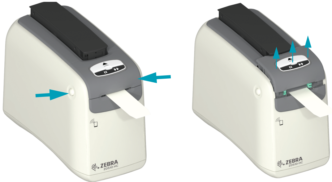
Figure 8 • Releasing Media Under the Upper Cover
